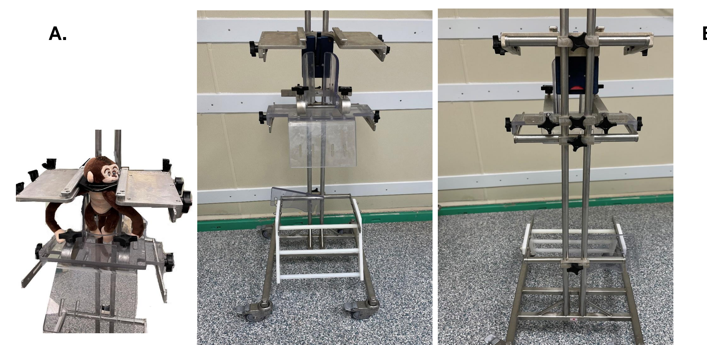
Figure 3. Restraint chair. A. Front B. Back Restraint chairs maintain an animal in a sitting position, with restraint being affected by pillory-type attachments at the neck. Insert Demonstration of use.
