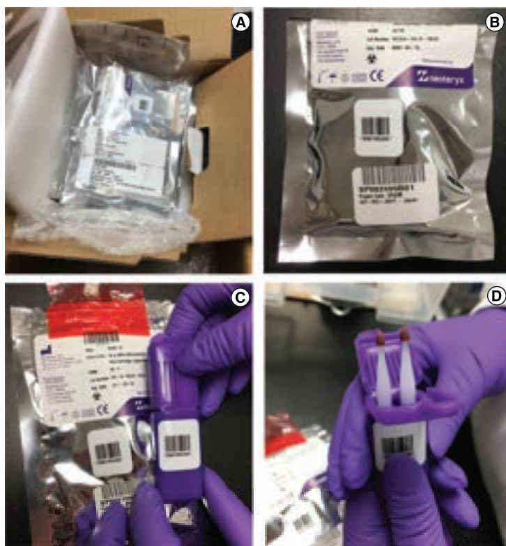
Figure 2. Clinical trial samples. (A) Mitra® volumetric absorptive microsampling (VAM) samples shipped ambient and received at the bioanalytical lab. (B) Mitra VAM cartridge packaged and secured inside the foil zip-lock bag. (C) Sample identification verified once the bag is opened at the bioanalytical laboratory. (D) Mitra VAM cartridge showing two tips with sampled patient's blood.
